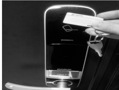
Figure 2. Door opening via smartcard
